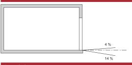
The illustrated maximum entrance angles must not be exceeded. Incorrect entrance angles will cause serious maneuvering and positioning problems on the parking system for which the local agency of INDAC Parking Systems accepts no responsibility.
