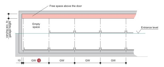
**12** GW = Grid unit width **must** strictly conform to dimensions quoted.
