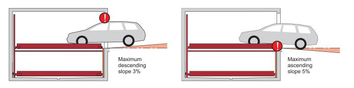
The illustrated maximum entrance angles must not be exceeded. Incorrect entrance angles will cause serious maneuvering & positioning problems on the parking system for which the local agency of INDAC Parking Systems accepts no responsibility.
